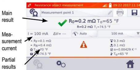
$R_0$  .....resistance at reference temperature
